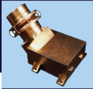
IES toroidal electrostatic analyser to measure ion and electron distribution functions
