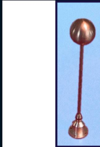
LAP spherical Langmuir probe, 5cm in diameter, made of titanium
